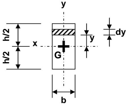
d'où  $\int_{-h/2}^{+h/2} y^2 \cdot ds = \int_{-h/2}^{+h/2} y^2 \cdot b \cdot dy = b \int_{-h/2}^{+h/2} y^2 \cdot dy = b \left[ \frac{y^3}{3} \right]_{-h/2}^{+h/2} = b \left[ \frac{(h^3/24)}{3} - \frac{(-h^3/24)}{3} \right] = \frac{b \cdot h^3}{12}$
