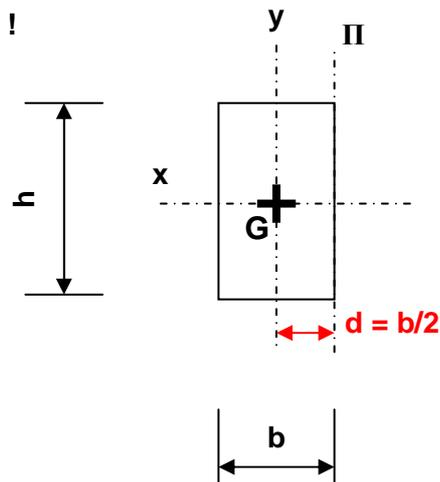
$$I_{II} = \frac{h \times b^3}{12} + \left[ \frac{b^2}{2^2} \times (b \times h) \right] = \frac{h \times b^3}{3}$$
